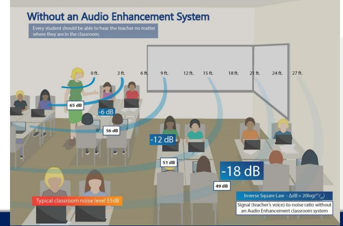
The *Inverse Square Law* states that as the distance doubles, the dispersing of a single source spreads over four times the area becoming only ¼ of its intensity. Just as you would not use one light bulb to illuminate a classroom, a teacher or student's voice is not a sufficient source of sound.
